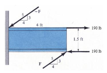
9. Replace the force at *A* by an equivalent force and couple moment at point *P*.
